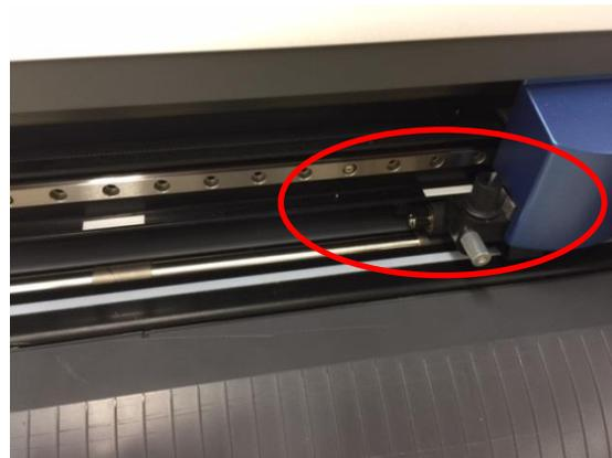
4. Lower the pinch rollers by *bringing the loading lever in the back UP*.
