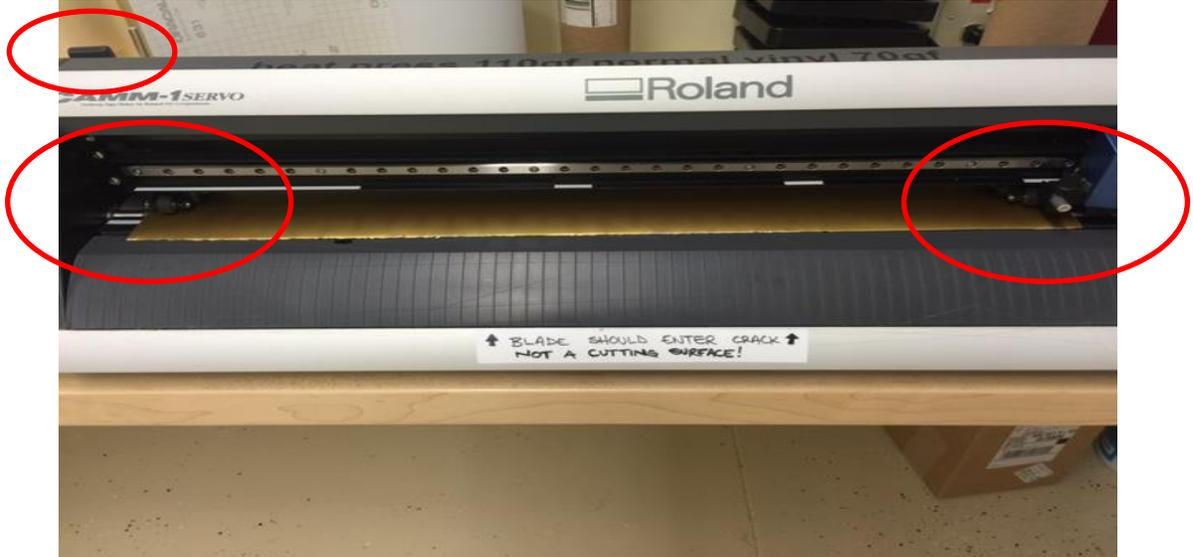
5. The display will ask you to “select sheet.” Choose “**roll**” by using the arrow buttons and then press the “**enter**” button. The blue cutting head will move all the way to the left and the width of the material will appear on the display in “mm” (ex: 561 mm).
